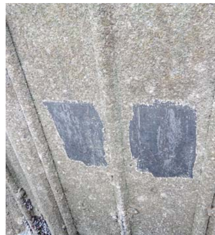
Intact PUR corrosion protection after 22 years
